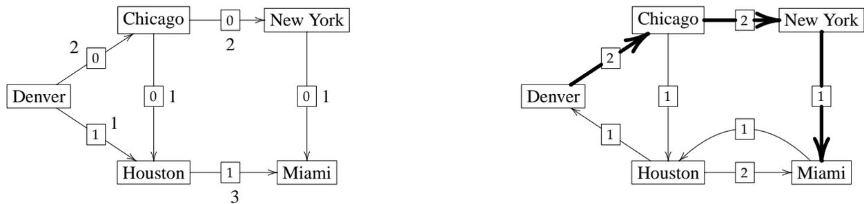
augmenting chain of residual capacity 1  $\rightarrow$  increase flow by 1
