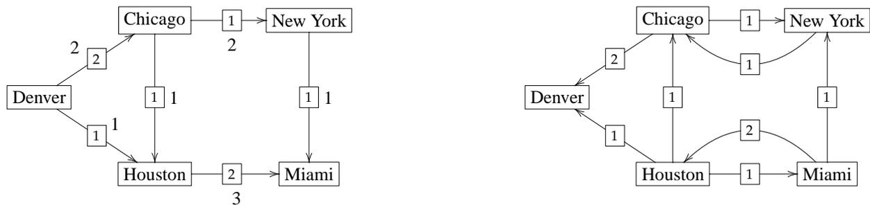
no path from Denver to Miami in the residual network  $\rightarrow$  no augmenting chain  $\rightarrow$  **optimal solution** found
